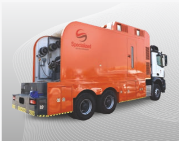
Open / Cased Hole Logging Truck Unit
